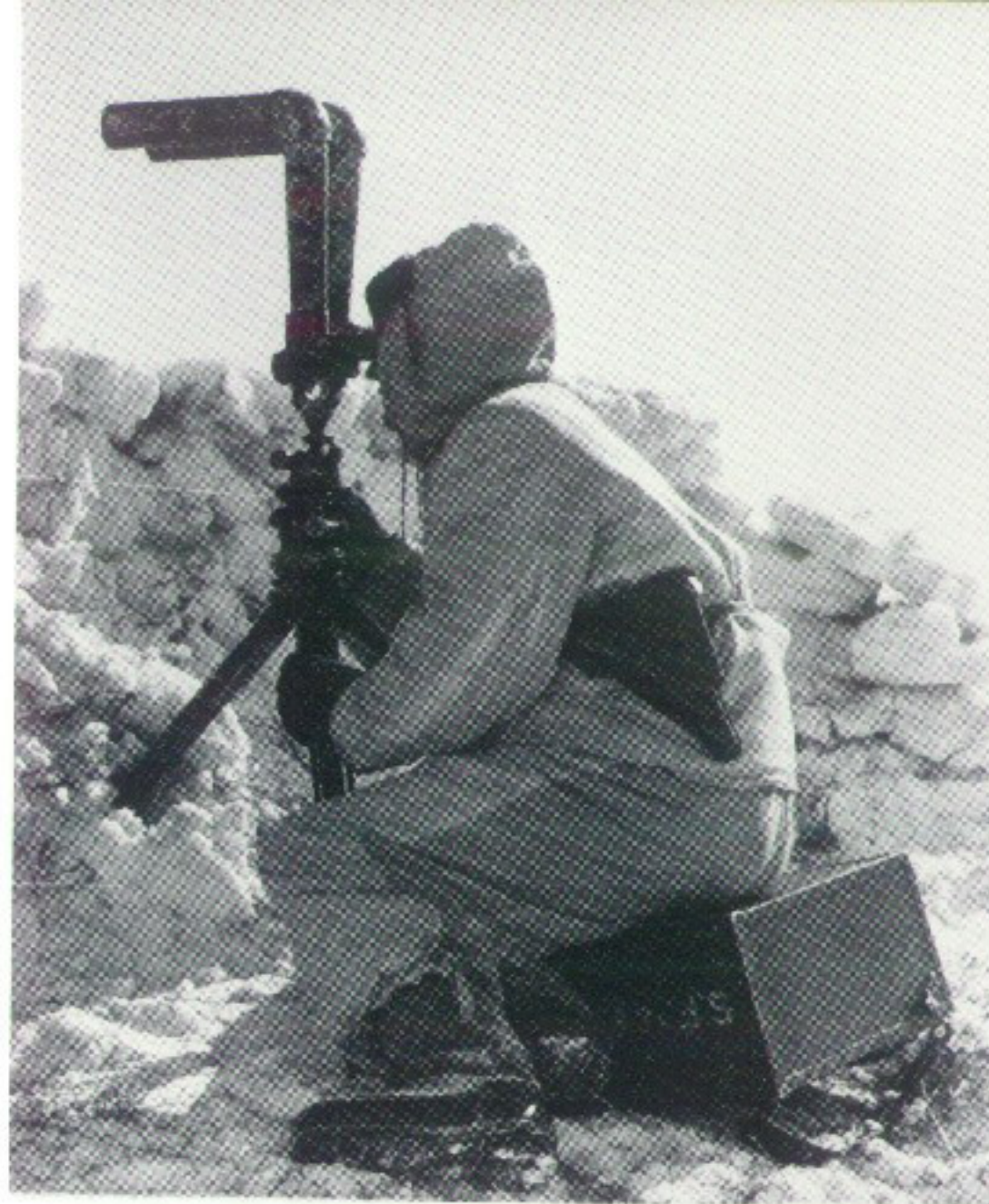
At a forward spotting position, a Panzergrenadier is seen using the standard binocular artillery spotting telescope. This device is fitted with extension tubes over the objectives in order to reduce snow glare. These were also often used in the desert to reduce glare from the sun. The wall of snow 'bricke' provides adequate camouflage from the enemy. (Bundesarchiv)
