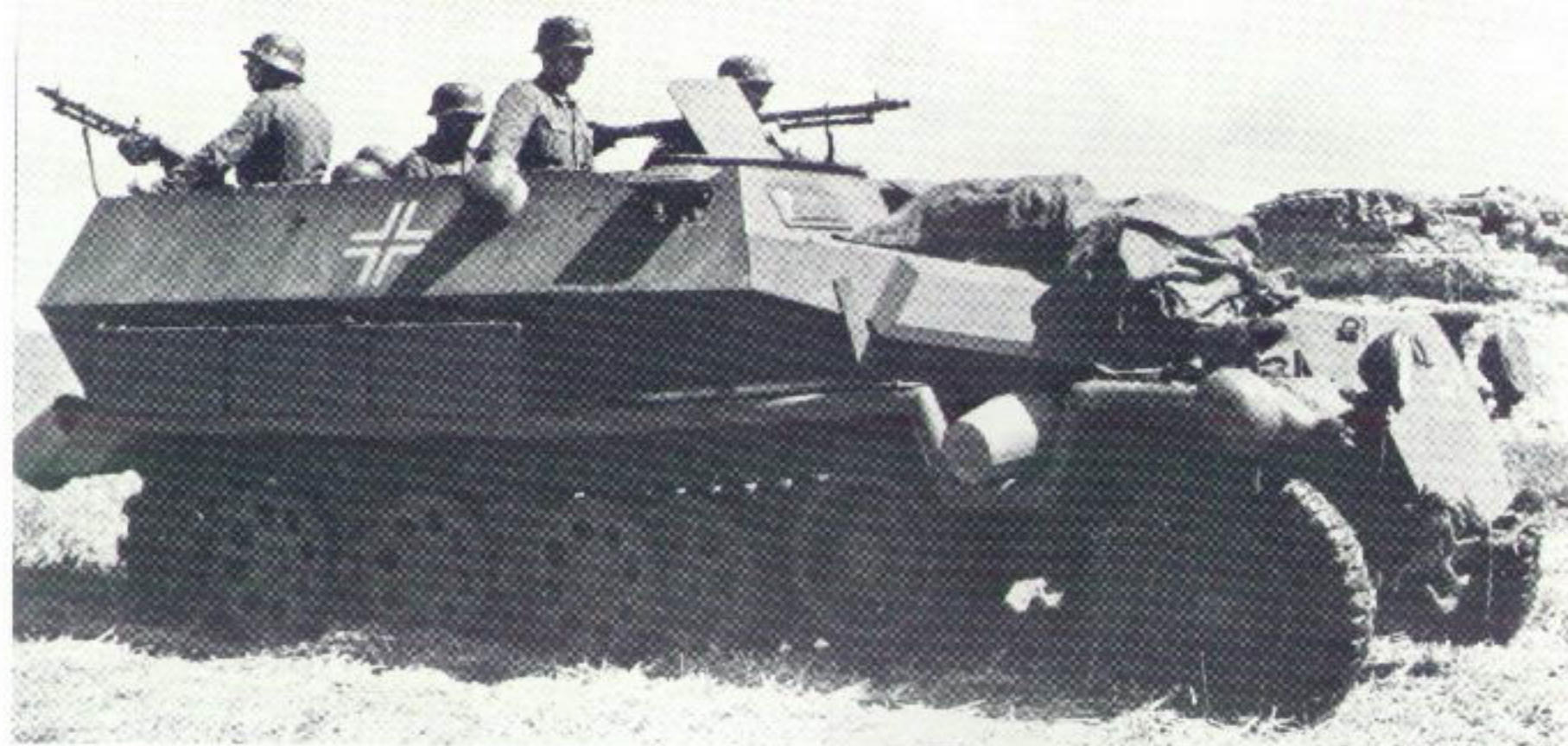
A Sdkfz 251 ausf C of the 14th Panzer Division is seen in Russia. The ausf C was the first model to benefit from combat experience, and featured a redesigned nose and cooling ducts for the engine. The forward MG 34 was used to support the crew of the vehicle, while the rear gun was intended for anti-aircraft use as well as for ground targets. (Bundesarchiv)
